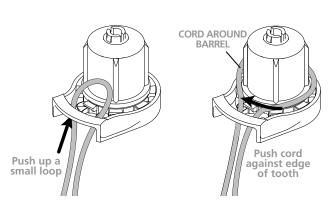
Push a loop up from behind the guard. Firmly push the cord clockwise against a tooth edge, until the pulley moves, trapping the cord in the pulley.
