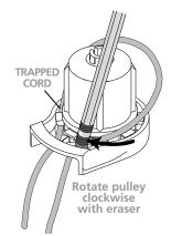
Use a pencil eraser to rotate the pulley clockwise, one tooth at a time, all the way around to the other side.
